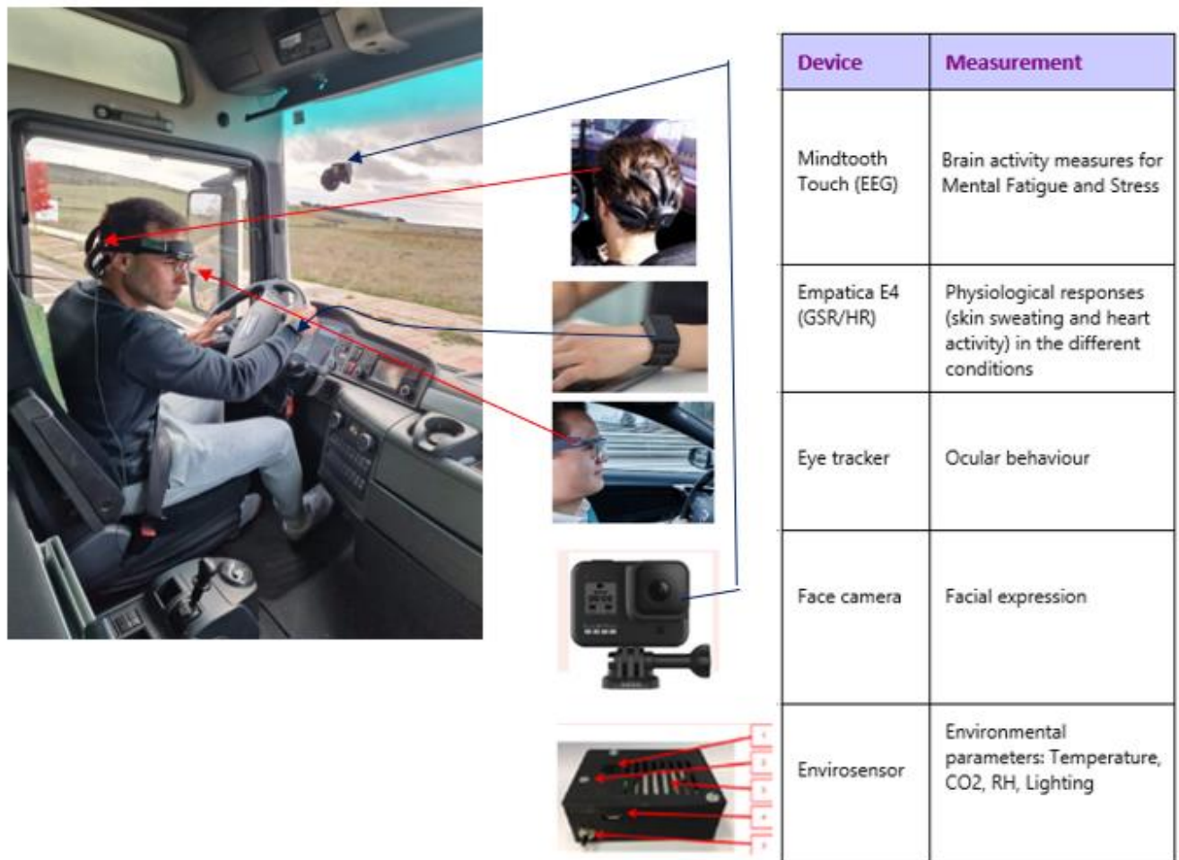
Figure 5: Devices for measuring the driver's neurophysiological data (picture taken during the C2 tests in Spain).
